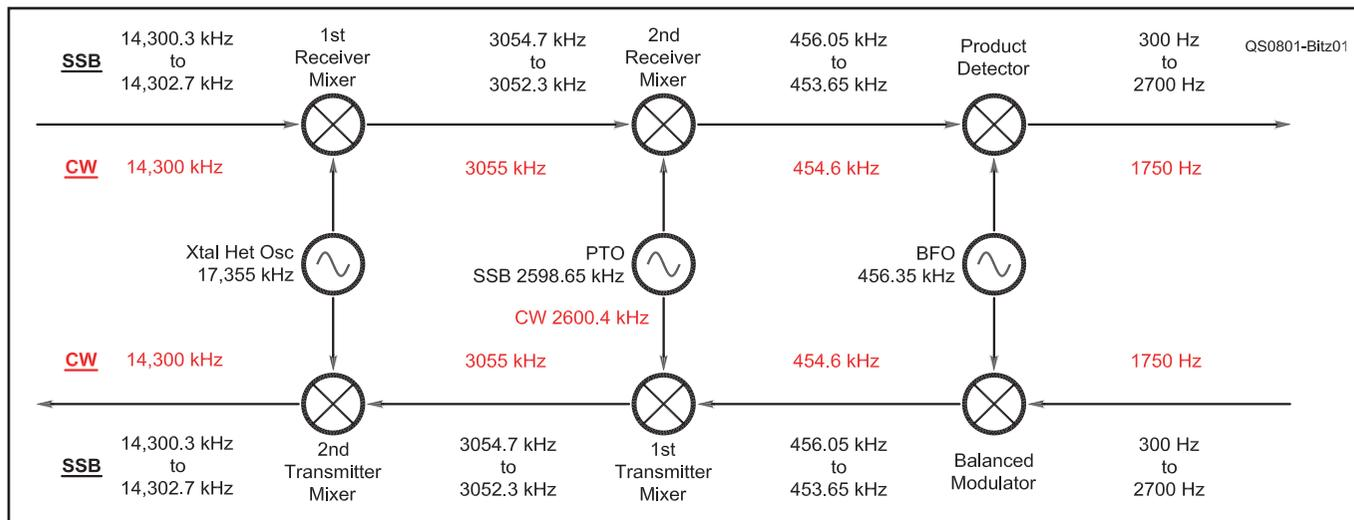
Figure 1 — The original KWM-2 frequency plan for SSB and CW modes.
