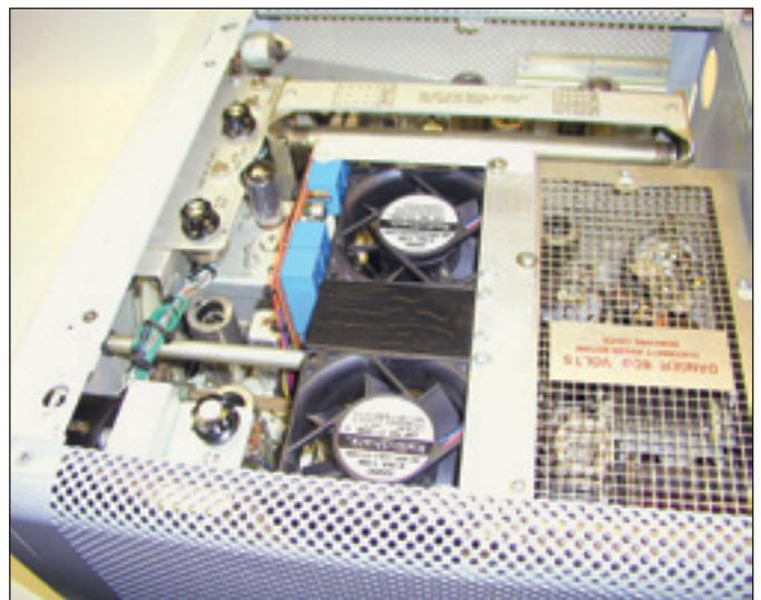
Figure 8 — Photo of the new KWM-2 BFO board in place behind PTO.
