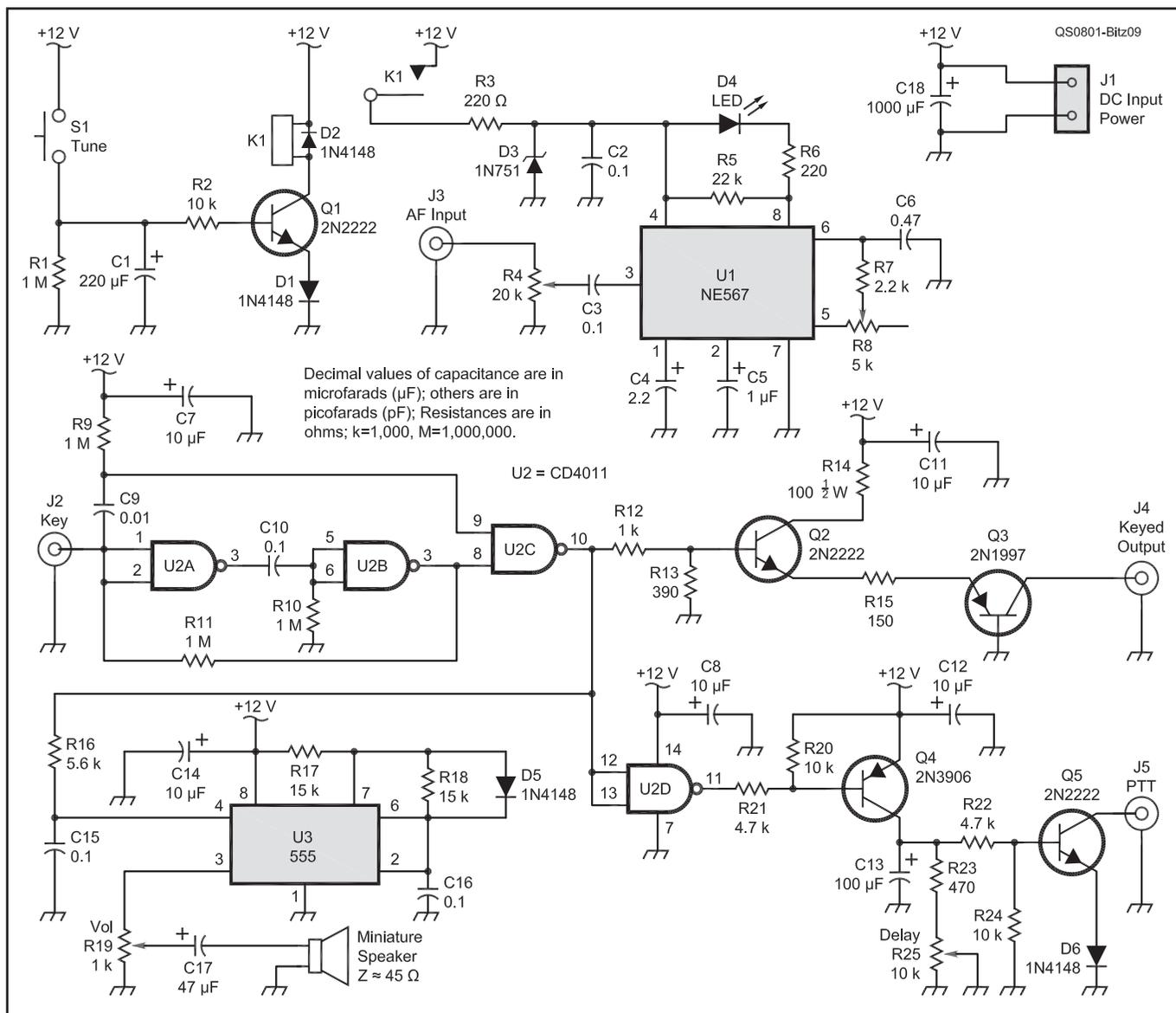
Figure 9 — Schematic diagram and parts list of external functions box.
