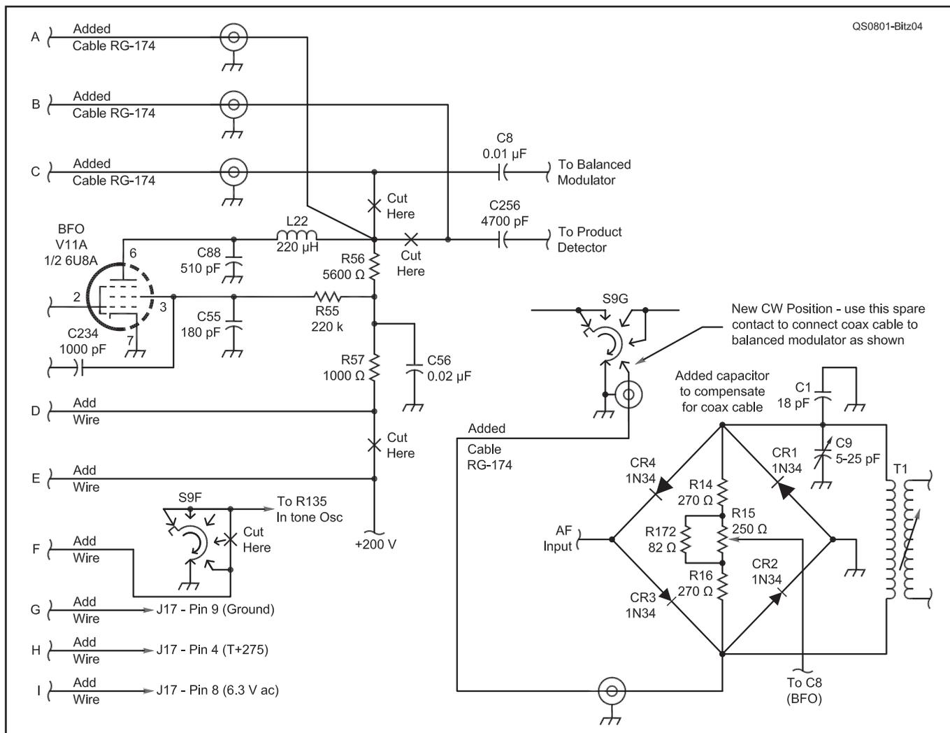
Figure 4 — Required KWM-2 circuit changes for CW modification. C1 is the only added part.
