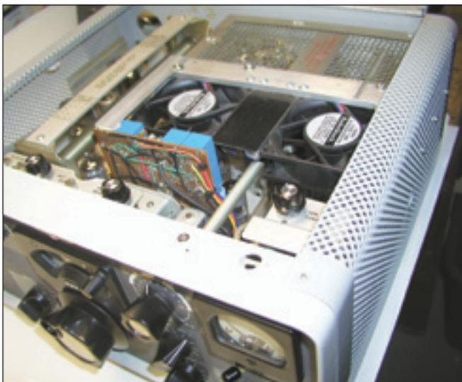
Figure 7 — Photo of the new KWM-2 BFO board being installed behind PTO. Cooling fans were added as a part of another project.
