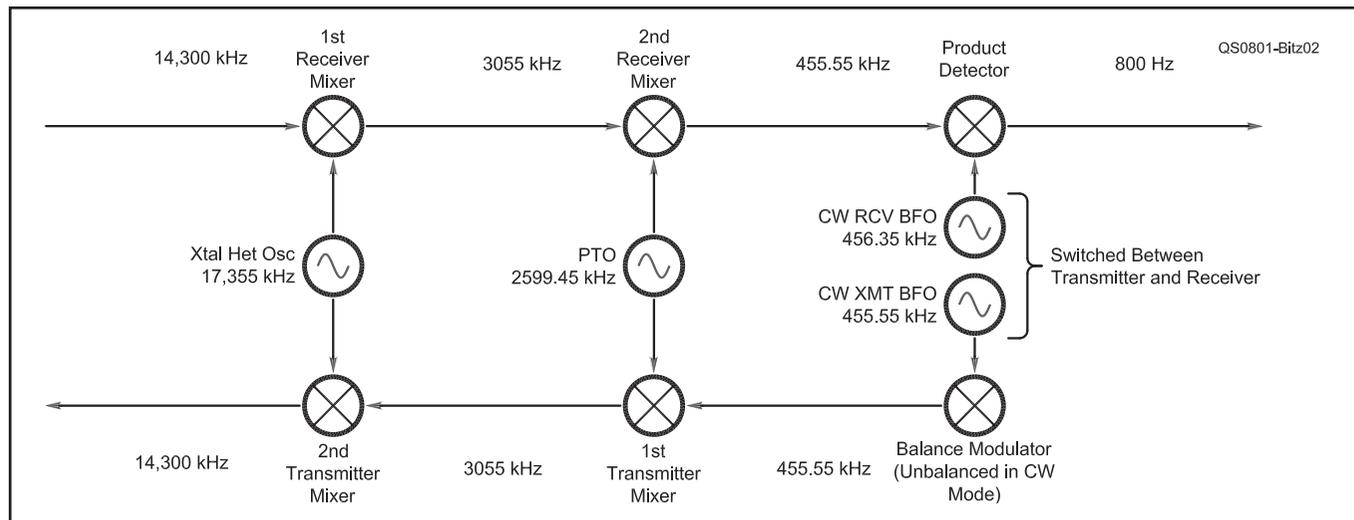
Figure 2 — Modified KWM-2 frequency plan for carrier generated CW operation.
