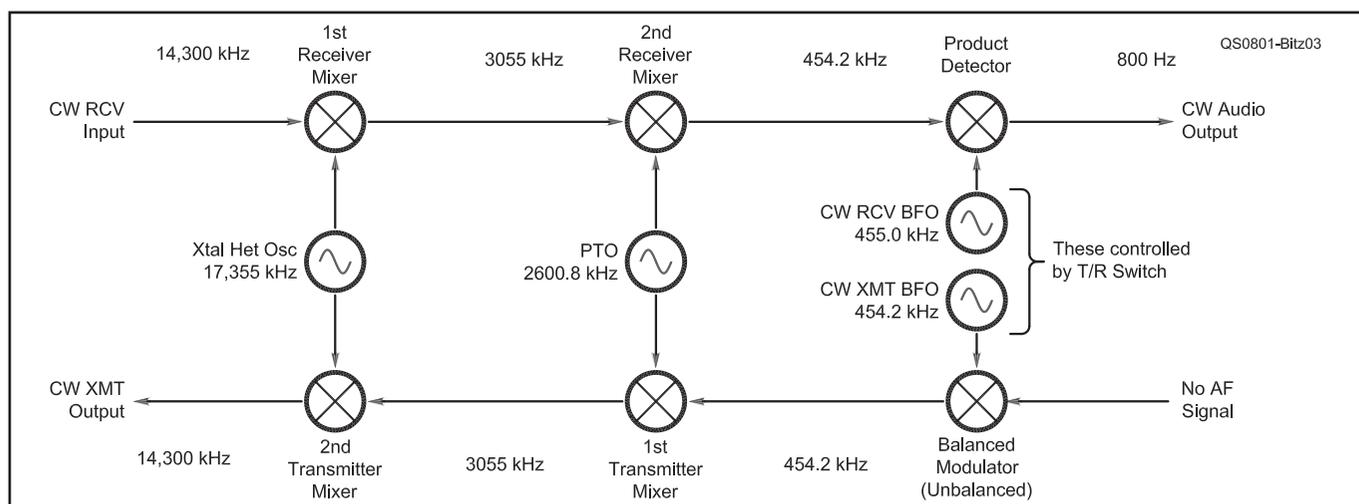
Figure 3 — Modified KWM-2 frequency plan for CW using two BFO frequencies.
